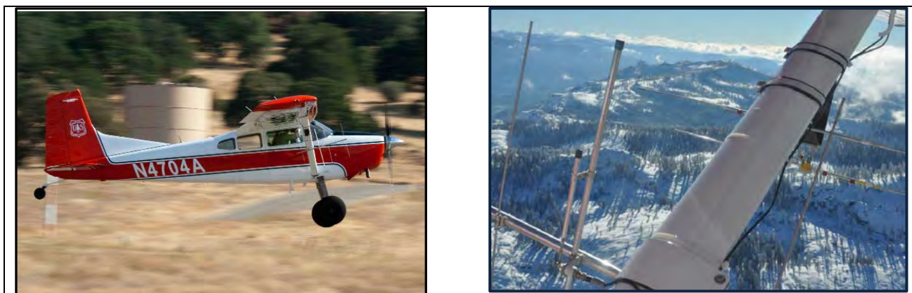
Illustration 7: Forest Service Cessna 185 airplane, and antenna configuration on the right side wing strut.
